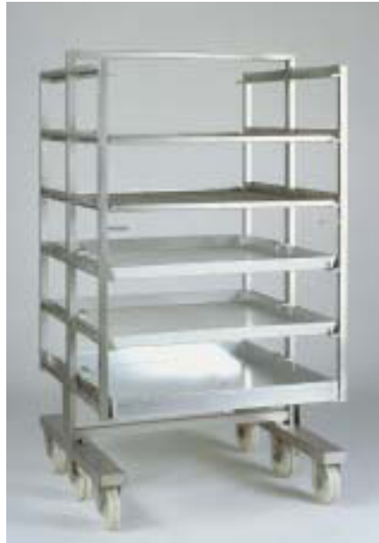
Truck for BASTRAMAT 850/851 Smoking stick length: 80 cm Supports: 5 / Support spacing: 25 cm External dimensions: 83 x 70 x 136 cm Floor clearance: 28 cm
