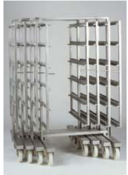
Truck for BASTRAMAT 1200/1201 Smoking stick length: 90 cm Supports: 5 / Support spacing: 25 cm External dimensions: 98 x 80 x 150 cm Floor clearance: 42.5 cm
