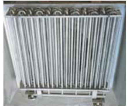
High-pressure steam register
